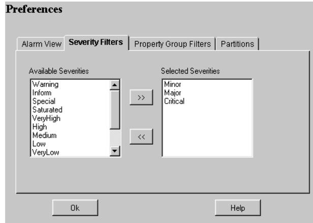
The first time you open it, the **Available Severities** list contains all the severities defined in the database of the first NerveCenter server to which you connected.
