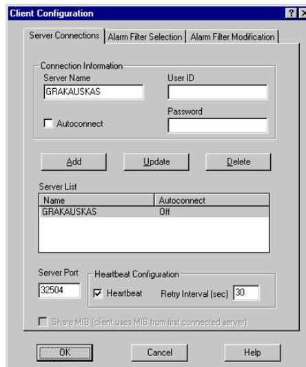
2. In the **Server List** near the bottom of the window, select the name of the server that uses the non-default port number.
