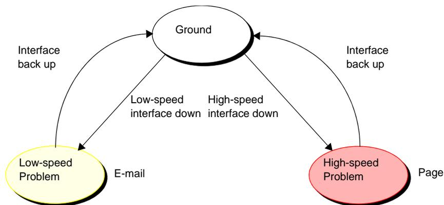
**FIGURE 2-2.** State Diagram for Detecting a Router Interface Problem
