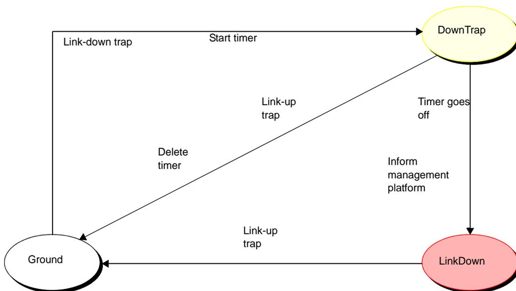
**FIGURE 2-1.** State Diagram for Detecting a Link-Down Condition
